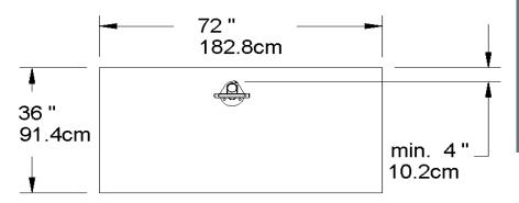
The minimum space requirements for High Security Bike Pumps are meant to allow a cyclist and their bike access to the pump.
